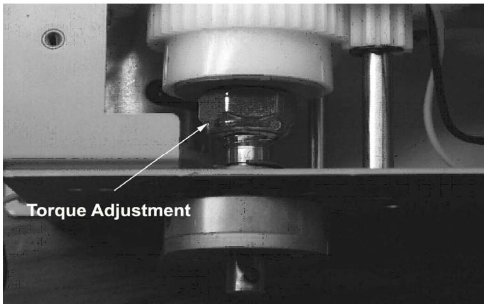
If you tighten the clutch enough to exceed the maximum torque rating, you may hear a loud clacking sound in the servo and the servo may disengage. This clacking happens when the force pushing the gears apart exceeds the solenoid's ability to hold the gear train engaged. This is a redundant safety feature – just back off on the control nut a little and recycle the power switch to re-engage the servo.
