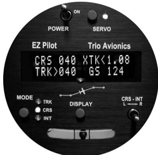
2. Going directly back to the **TRK** mode causes the EZ Pilot to more gradually curve back to the **DTK**.
