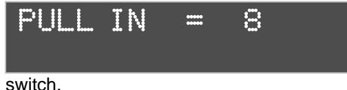
Here again, pressing the **MODE** switch will replace the equal (=) sign with an arrow and allow the value to be changed using the **L-R** switch.
