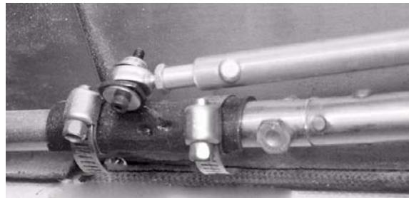
It will simplify installation adjustments if there is enough overhead clearance to allow removal and replacement of the servo lid with the servo remaining in place (for instance, you will possibly want to adjust the slip clutch). The servo lid is secured by two screws on the top of the lid.
