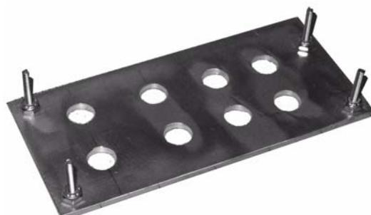
mounting tabs will fit down over the screws. Nuts can be tightened down to secure it. For a composite aircraft installation, the bottom of the plate (shown above) should be floxed and the holes in the plate filled with flox before applying fiberglass layers over it to secure it to the fiberglass structure.
